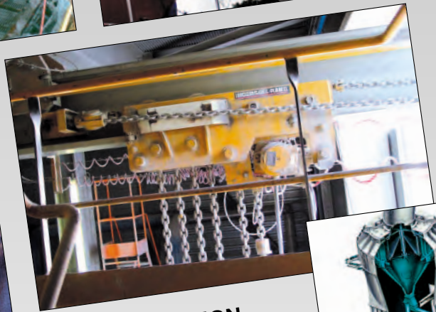
COMPACT DESIGN Air or hydraulic chain hoists brings strength and durability to maintenance operations in cement plants: replacement of milling wheels.
