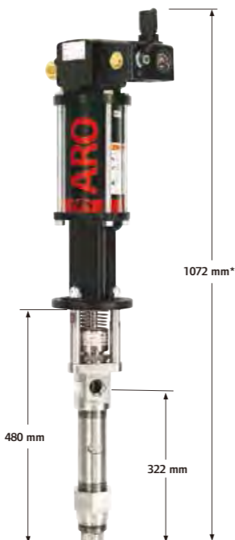
Model shown w/ball valve regulator *For models without ball valve regulator subtract 52.83mm
